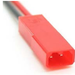
Figure 7. Team-provided connection to the manual shutdown interface
