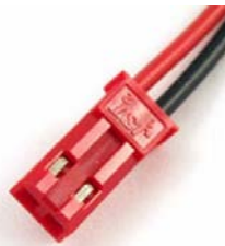
Figure 8. Competition-provided connector for manual shutdown interface
