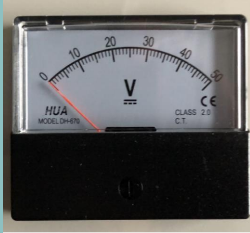
Figure 5: Hard-wired Voltage readout
