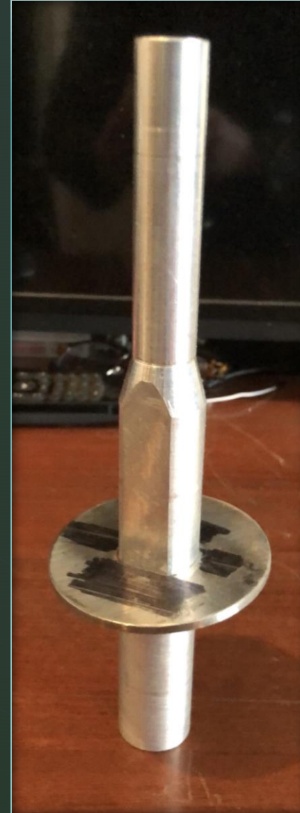
Figure 13: Partially Machined Shaft and Disk
