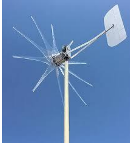
Figure 10: Small single yaw system[Y1]
