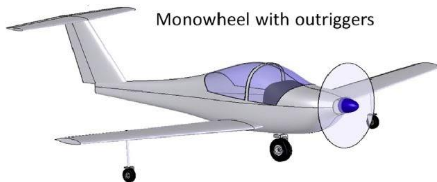
Figure 8: Monowheel with Outrigger Landing Gear Configuration [30]
