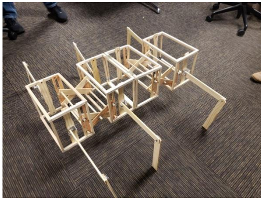
Figure 40. Wooden prototype extended body segment mode.
