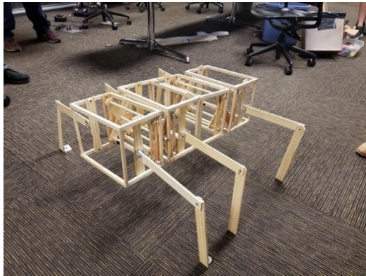
Figure 41. Wooden prototype contracted body segment mode.
