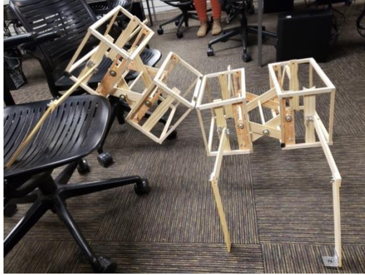
Figure 39. Wooden prototype climbing mode utilizing midbody hinge.
