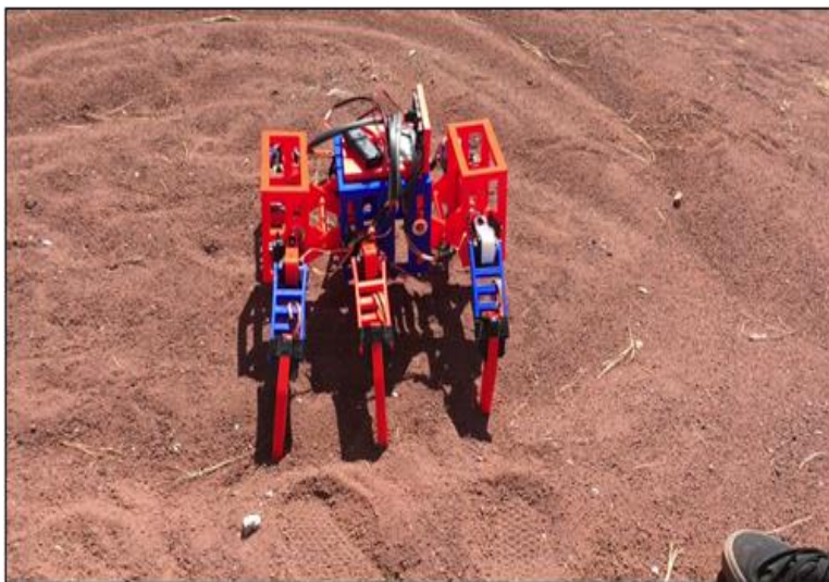
Figure V. Image of Small-Scale Model walking on sand
