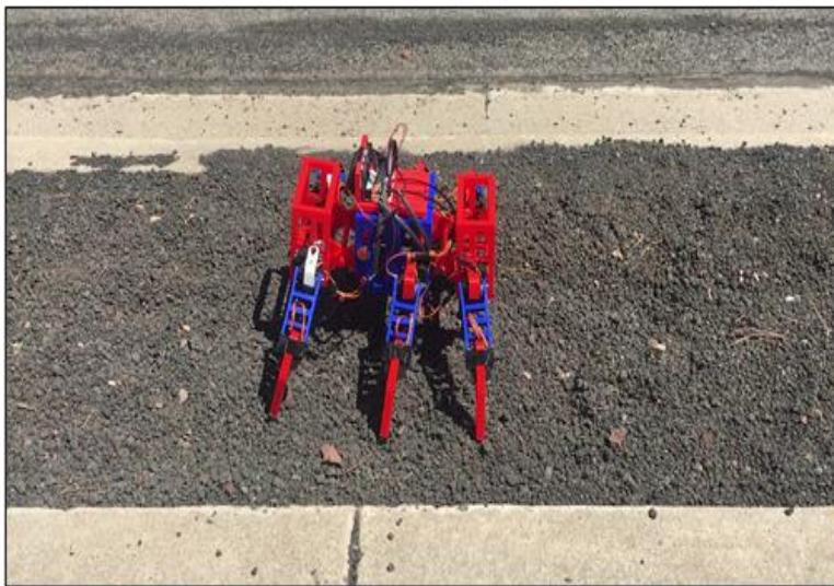
Figure IV. Image of Small-Scale Model walking on gravel
