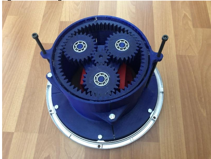
Figure 3. Full-scale leg model base planetary gear box.
