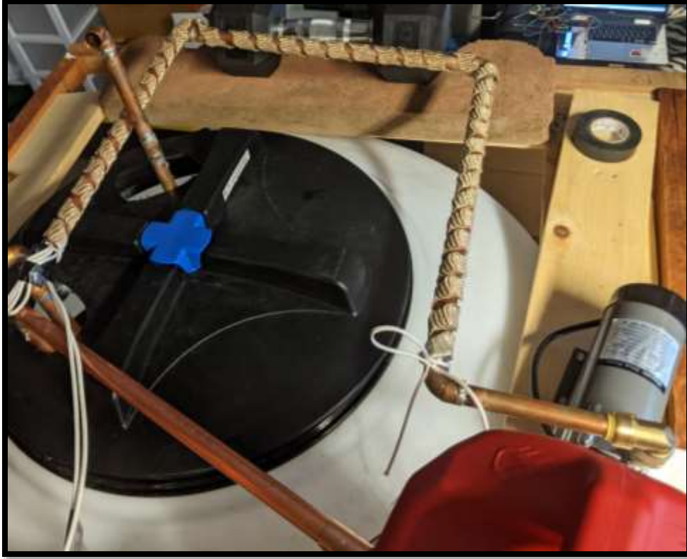
Figure 14: Heating tape wrapped around copper piping.
