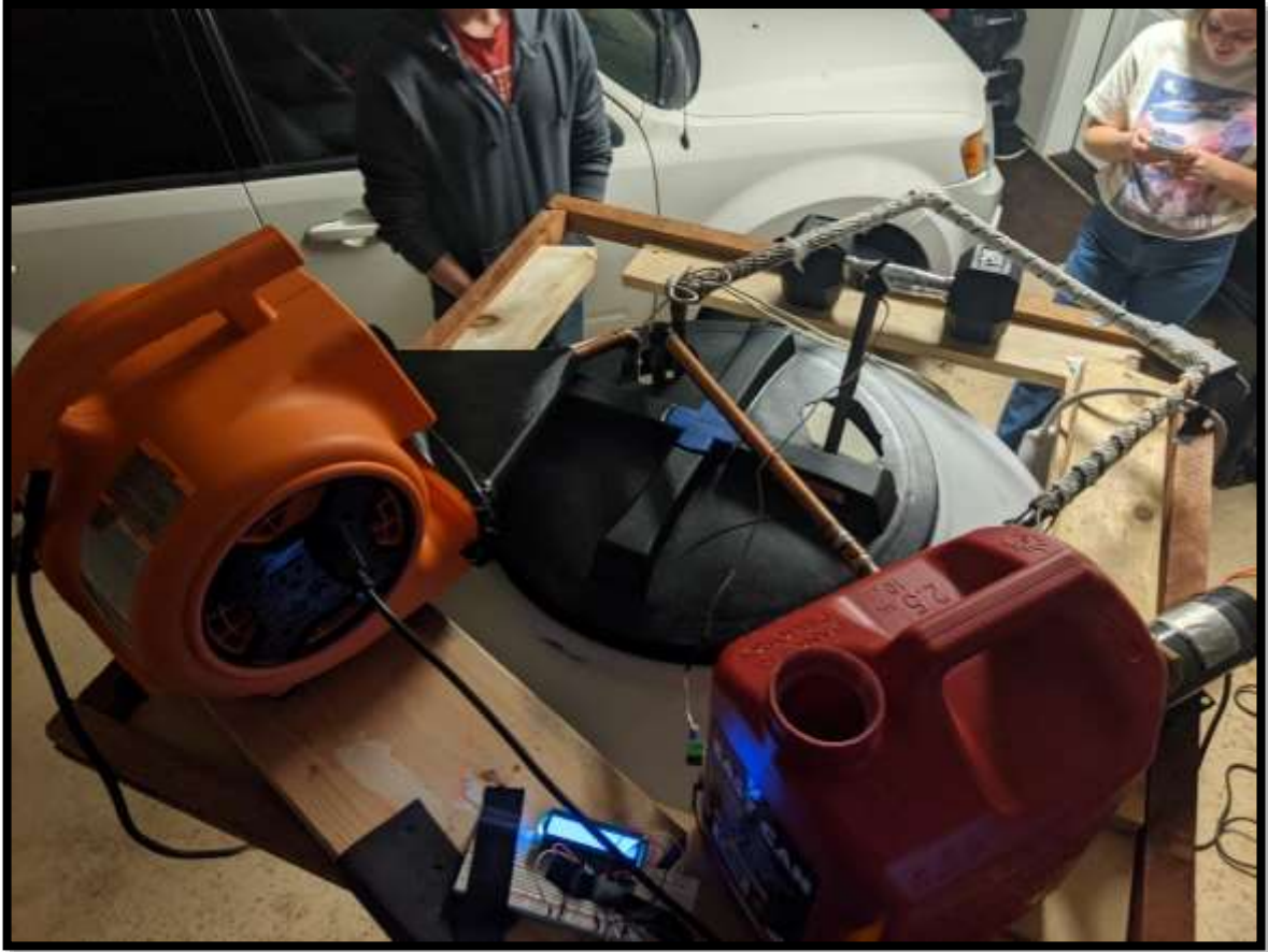
Figure 9: Component placement on platform with Arduino and heating tape
