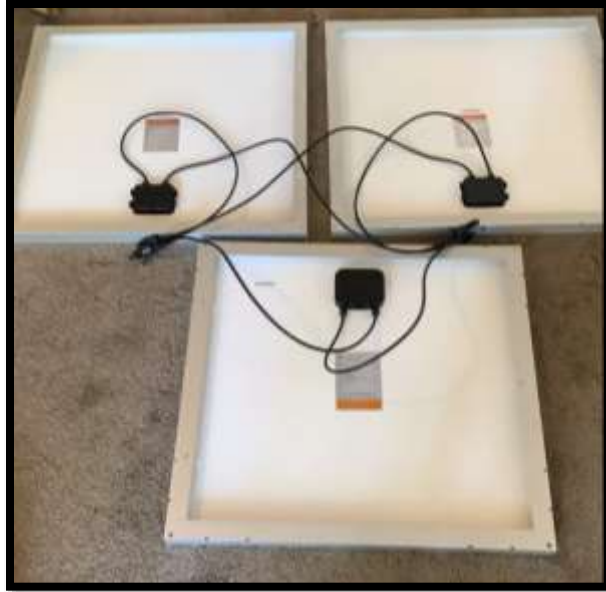
Figure 15: Solar PV Panels parallel setup
