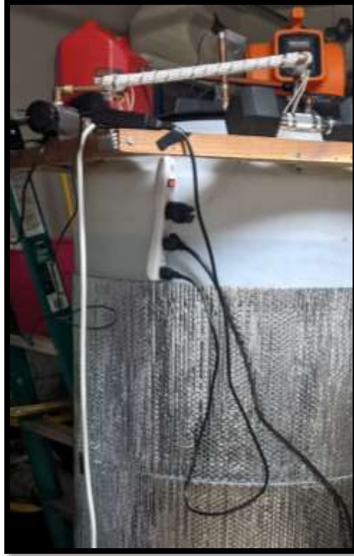
Figure 18: The electrical plugs for the heating cycle
