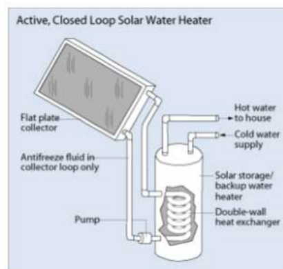
Figure 5: Indirect System with Active Circulation [9]
