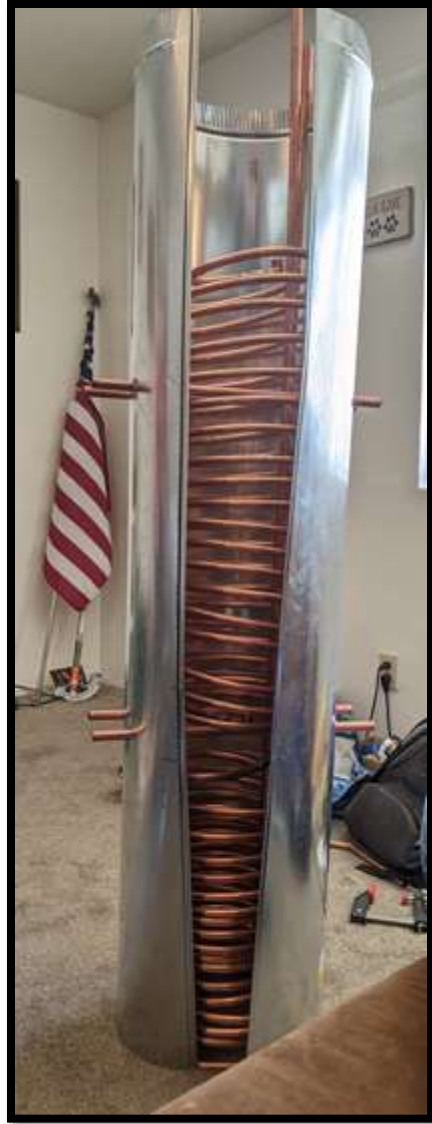
Figure 17: Heating duct with heat exchangers inside of it
