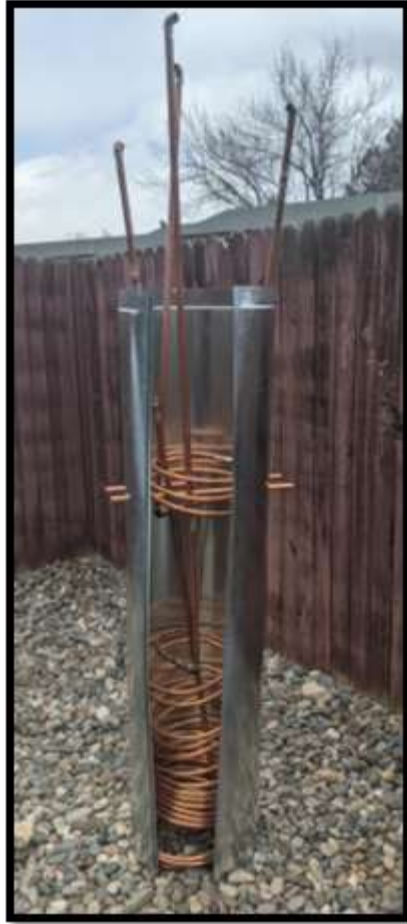
Figure 18: Heat exchanger ducting with smaller heat exchanger
