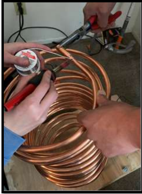
Figure 16: Heat Exchanger Coiling and Soldering
