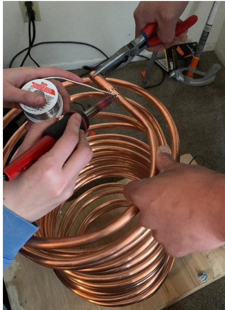
Figure 1: Heat Exchanger Coiling and Soldering
