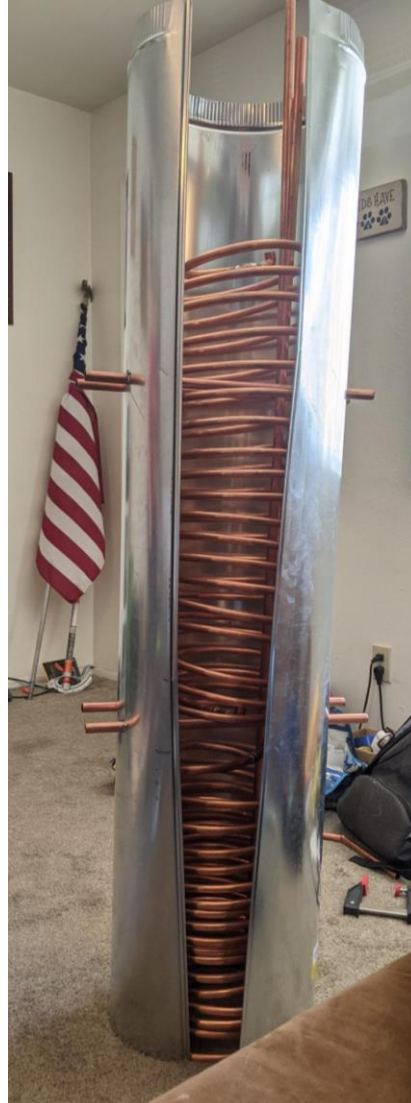
Figure 2: Heating duct with heat exchangers inside of it
