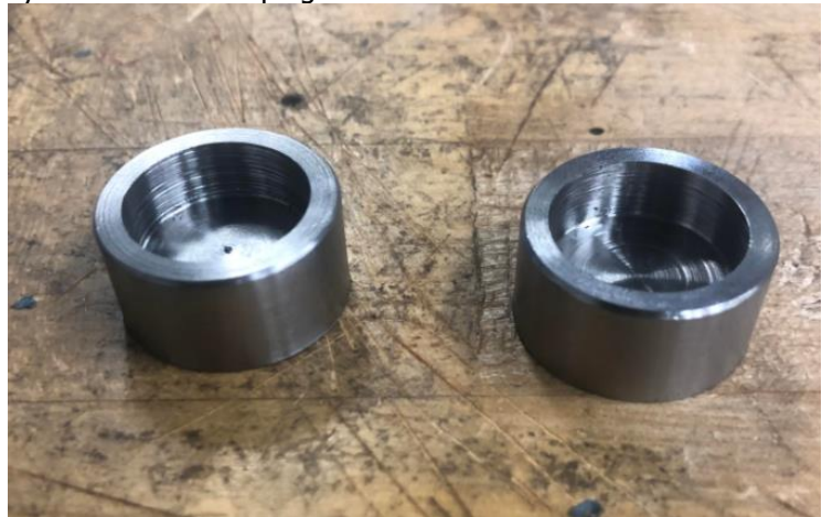
On the inside of the exterior brake caliper body, two cylindrical titanium plugs were machined out of titanium.
