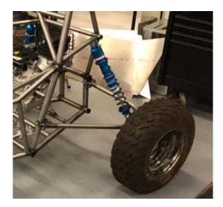
Figure 33: Rear Suspension Mockup
