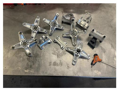
Figure 19: More Rear Hub and Pillow Block Bearing Clamps
