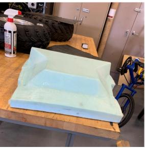
Figure 2: CNC Machined Fiber Glass Hood
