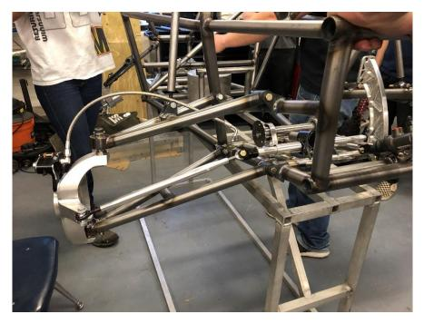
Figure 27: Front End Assembly
