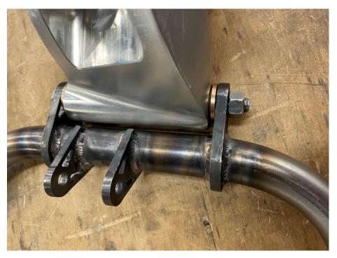
Figure 30: Knuckle mounting Tabs
