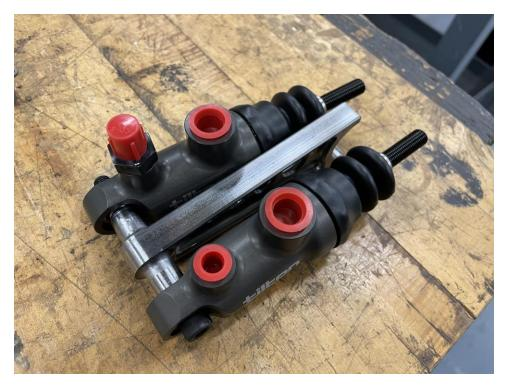
Figure 11: Master Cylinder Mount machined from 4130uyb
