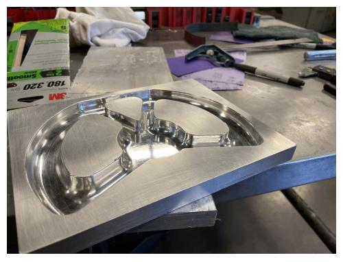
Figure 8: Steering Wheel Mold
