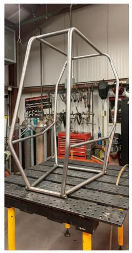
Figure 1: Isometric view of Primary Members tack-welded together
