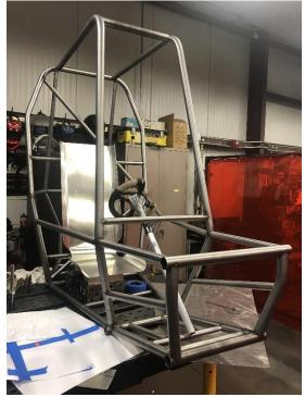
Figure 6: Front View of Frame with Complete Roll Cage and Front Members
