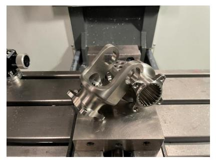
Figure 12: U-joint yokes machined from titanium
