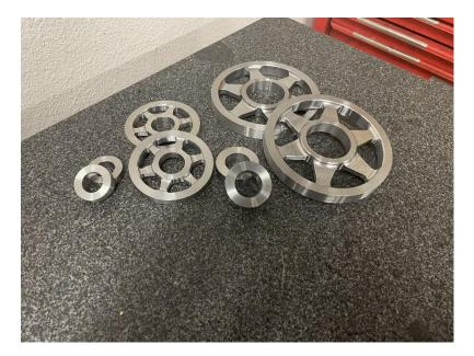
Figure 13: Gear Blanks Machined from 9310
