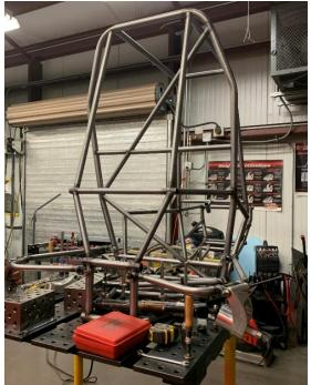
Figure 3: Rear-View of Chassis, Rear-End Shock Member
