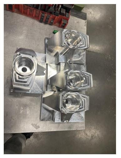
Figure 10: Front Upright's Left and Right Sides
