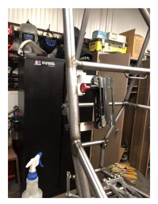
Figure 7: Fire Extinguisher Mount
