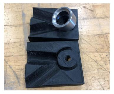
Figure 23: 3D Printed A-arm Jigs
