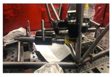
Figure 32: Frame Mounting Sleeve Hole Saw Jig
