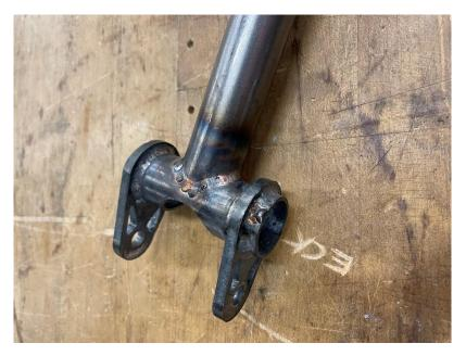
Figure 31: Rear Arm Knuckle Mounting Tube/Tabs
