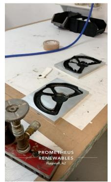
Figure 4: Nova Kinetics Facility, Steering Wheel Pre-preg Lay-out
