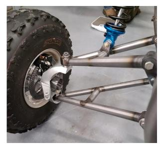
Figure 28: Passenger Side Knuckle
