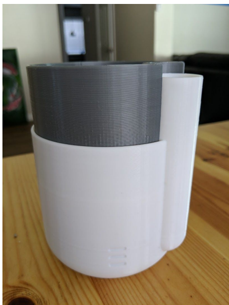
Figure A4: 2 pieces self-watering planter printed at 0.2mm layer height, 3 walls, no infill
