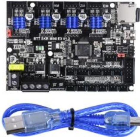
Figure A1: SKR E3 mini Circuit board upgrade
