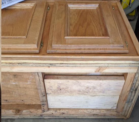
Figure 2: 2x6 Bottom reinforcement
