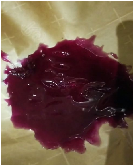
Figure 1: The melting plastic after heating it inside the oven in 215.5 celsius.
