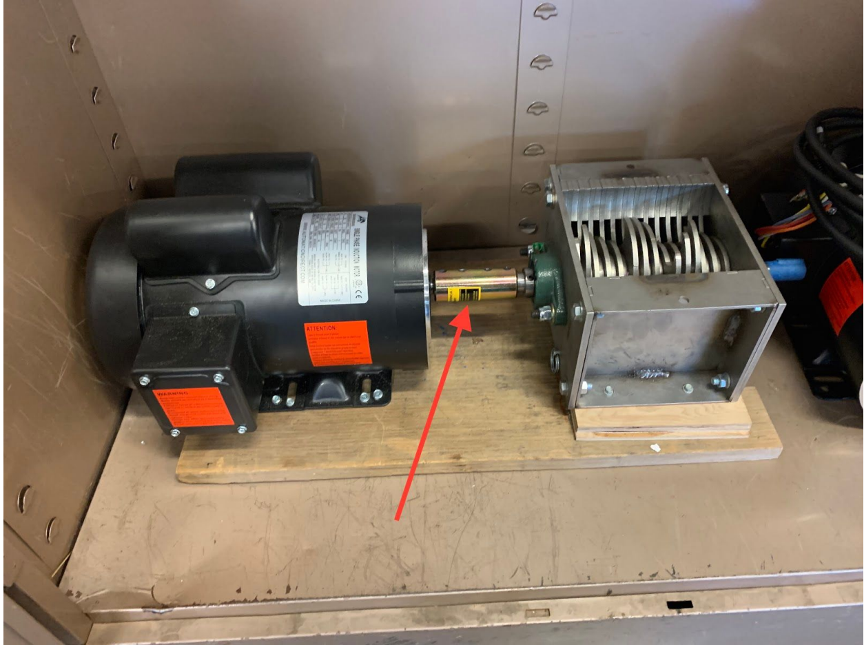
Figure 5: The coupler attached between the shredder and the motor
