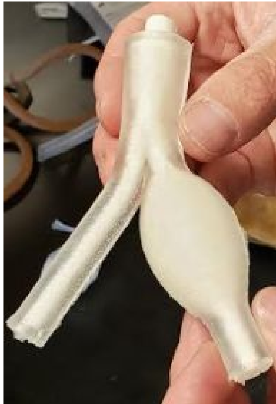
Figure 26. Prototype Iliac Bifurcation Model Proving a Successful Manufacturing Process
