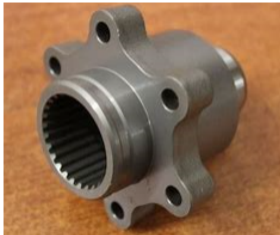
Figure 1. Rear Differential Output Flange (unmodified)
