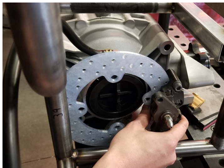
Figure 10. Expected rear brake setup and position
