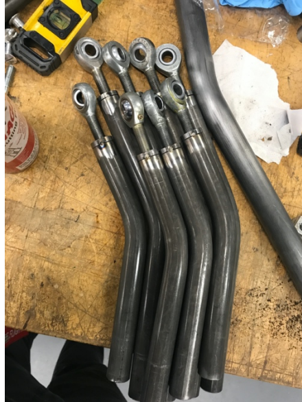
Figure 13. The rod end fitting design for the front end control arms
