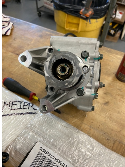
Figure 2. Modified Rear Differential Output Flange
