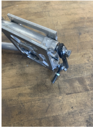
Figure 15. Weld Plugs on Prototype (Final Design)
