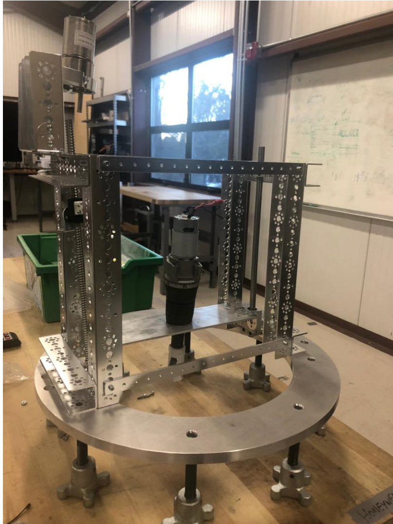
Figure 1: Full Mainframe & Base System with Drill Holder Plate and Torque Motor
