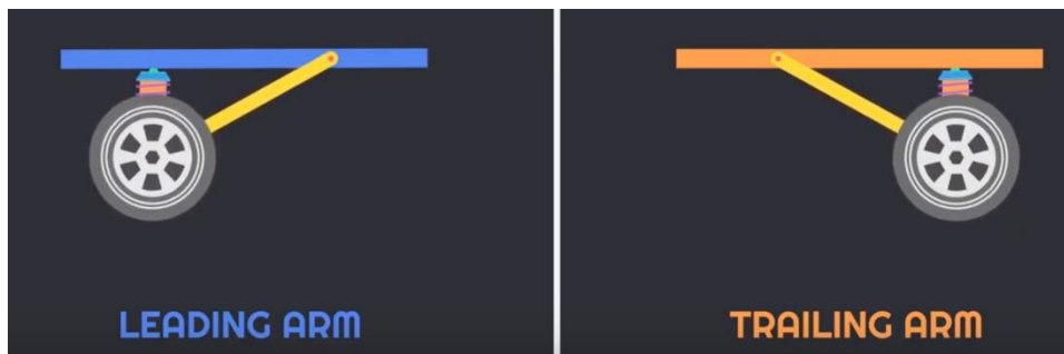
Figure 6: Trailing Arm vs. Leading Arm Diagram
