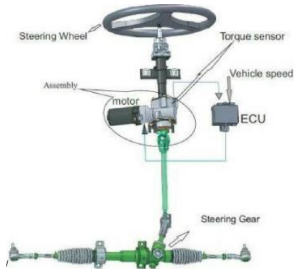
Figure 13: Electric Power Steering Setup [30]
