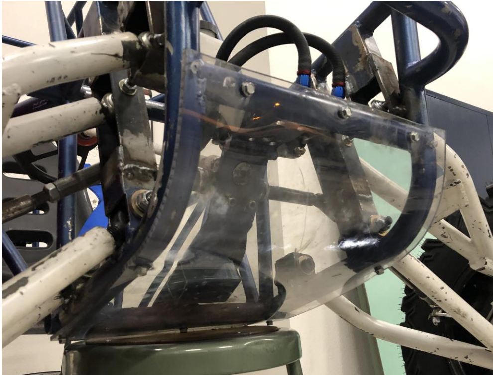
Figure 14. Clear skid plate addition
