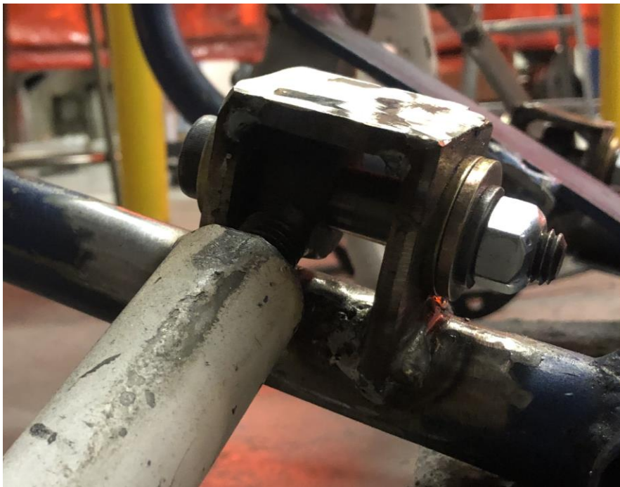
Figure 9. Front suspension welds
