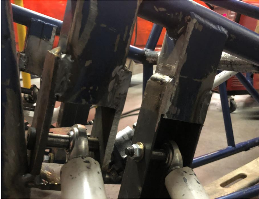
Figure 8. Front suspension welds
