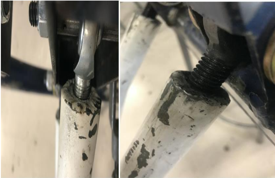
Figure 3. Tapped arm for the new joints
