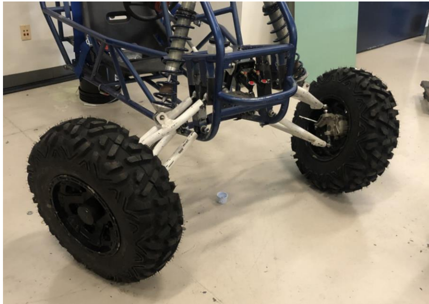
Figure 12. Unaligned front suspension
