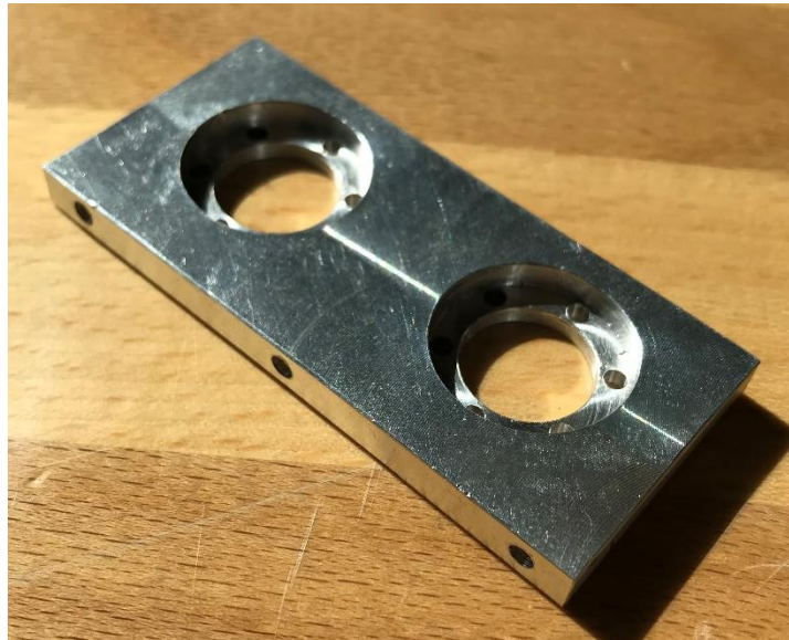
Figure 1: Motor mount cut on a CNC mill
