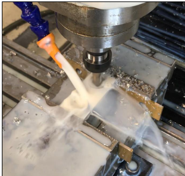
Figure 1.2: Finishing a Part on a CNC Mill
