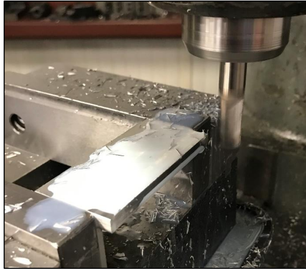
Figure 1.1: Roughing a Part on a Manual Mill
