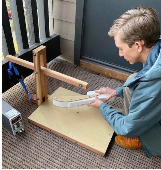
Figure 10: Homemade Hot-Wire Cutter in Use
