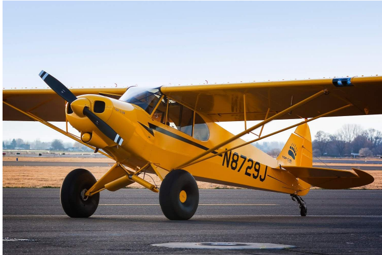
Figure 13: Conventional (Taildragger) Landing Gear on a Piper J-3 Cub
