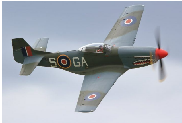
Figure 8: Tapered Wings on the P51 Mustang
