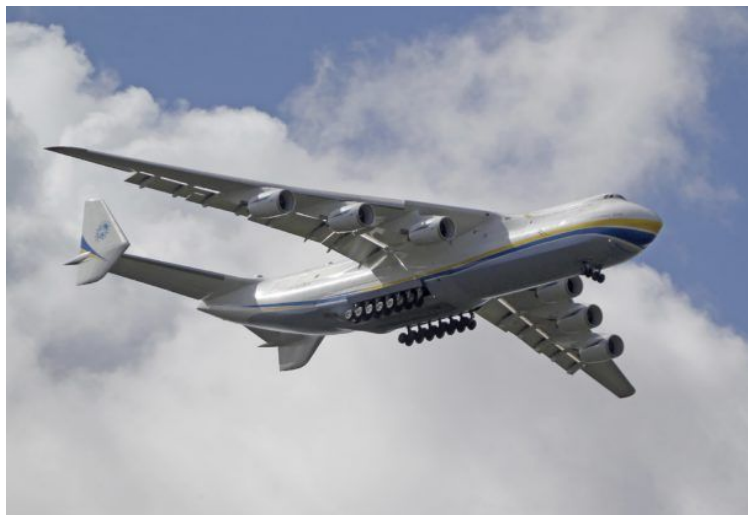
Figure 14: Tandem Landing Gear on an Antonov AN225
