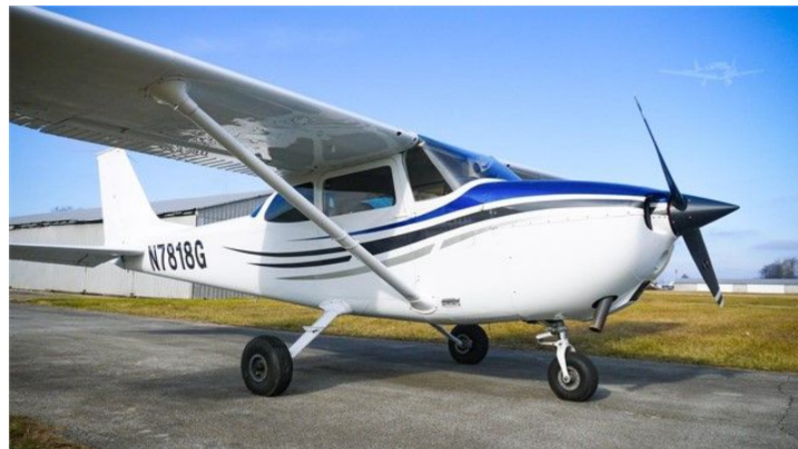
Figure 12: Tricycle Landing Gear on a Cessna 172
