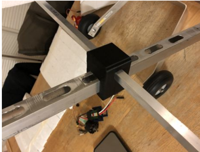
Figure 3: 3D Printed Connection Block
