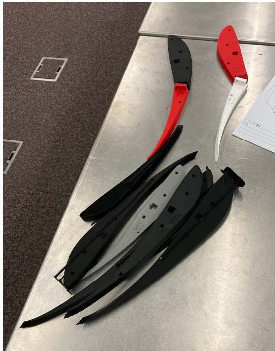
Figure 9: Varying Sizes of Wing Templates for a Tapered Wing
