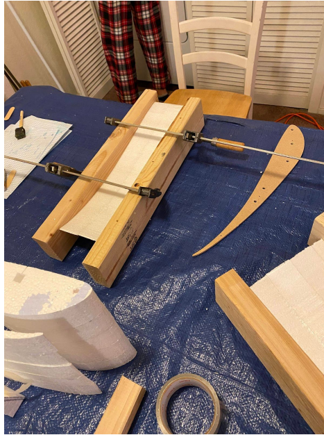
Figure 10: Clamping Together Cut Foam Wing Sections.
