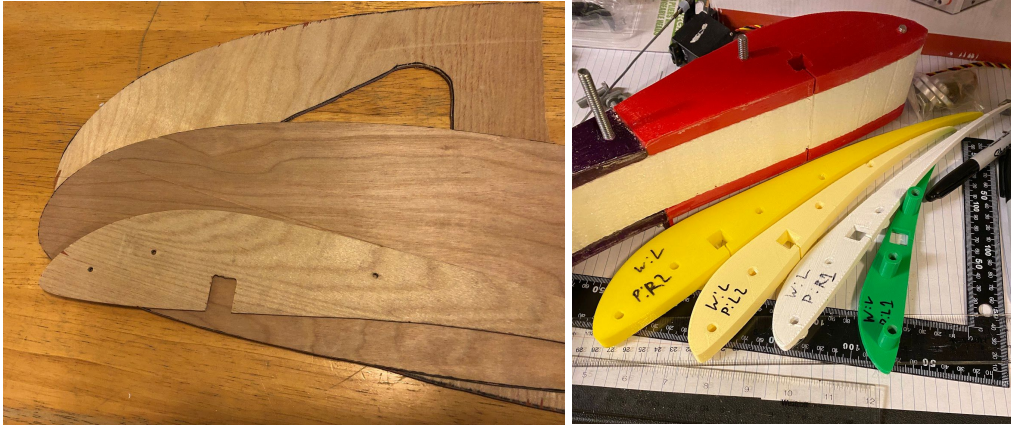
Figure 4: Wooden Templates (left) and 3D-Printed Templates (right)
