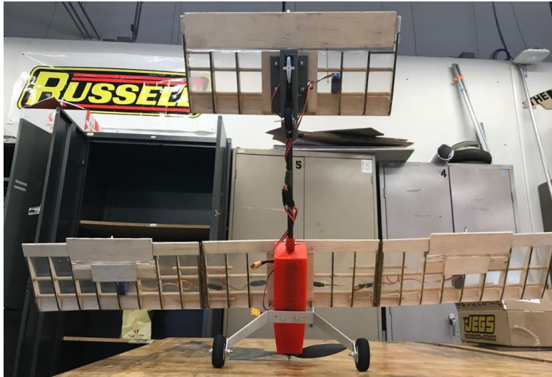
Figure 3: Oversized Landing Gears with Bolted Connections
