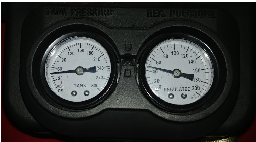
Figure 10: Compressor Pressure Gauge
