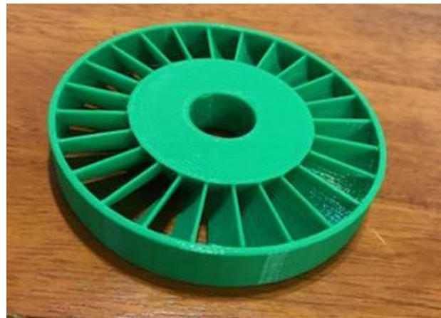
Figure 29: Second Stator Section
