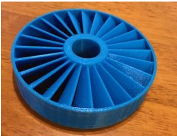
Figure 28: First Stator Section
