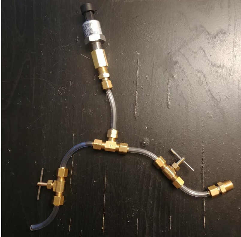
Figure 33: Pressure Measurement Manifold
