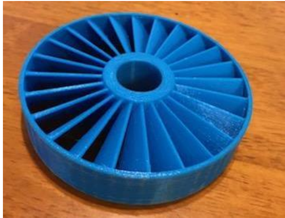
Figure 30: First Stator Section
