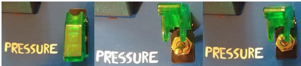
Figure 56: Turning on Pressure Measurement System
