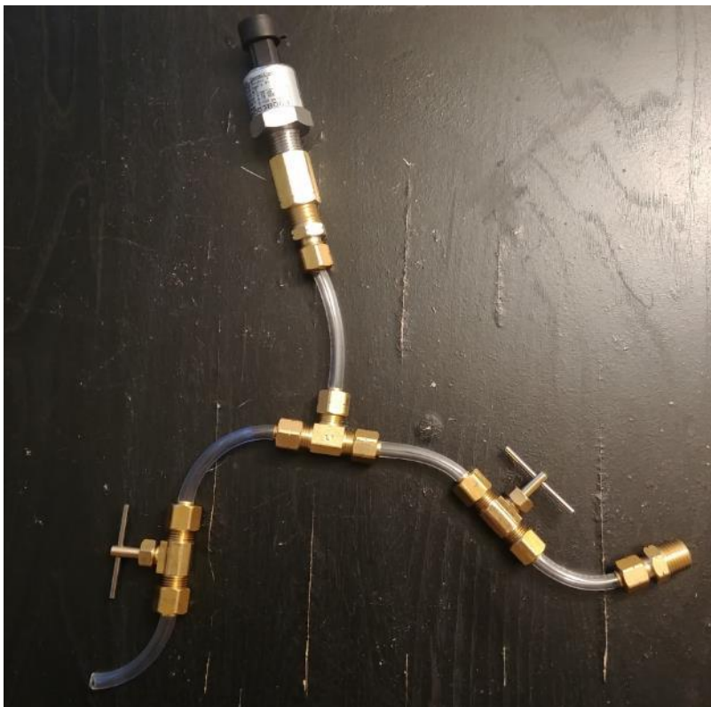
Figure 35: Pressure Measurement Manifold
