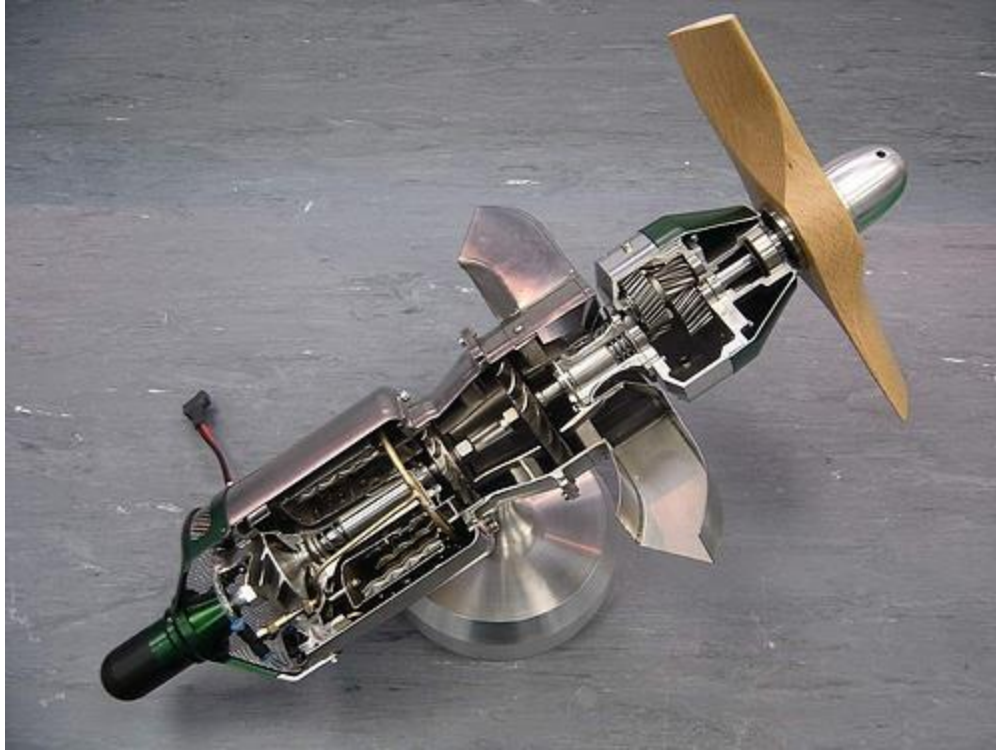
Figure 5: Wren 54 Turboprop Cutaway [4]
