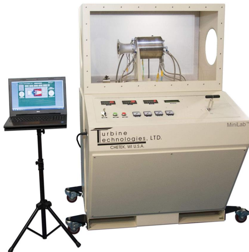
Figure 3: MiniLab Gas Turbine Lab [3]
