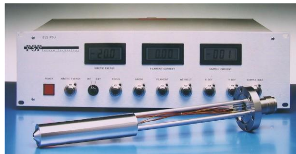
Figure 3.4.6: Electron Source ELS100 [9]
