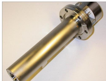
Figure 3.4.4: Flood Gun FS 100 [7]
