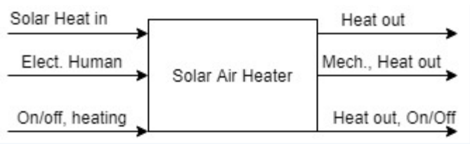
Figure 3: Black Box Model of the Solar Air Heater
