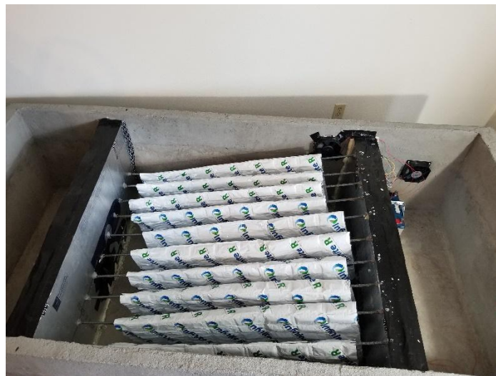
Figure 22: PCM Rack inside Thermal Box
