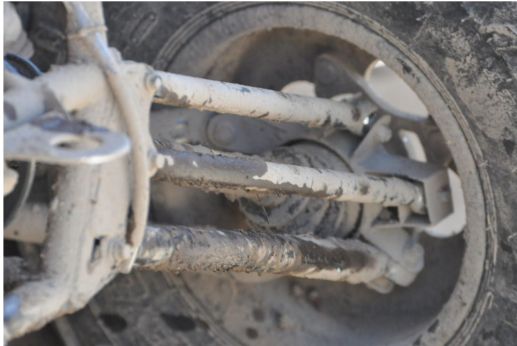
Figure 15: SDSU's 3-link system(Credit: Marco Sliva)
