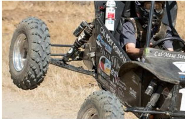
Figure 11: Cal Poly Baja - Trailing Arm Mounted Shock [5]
