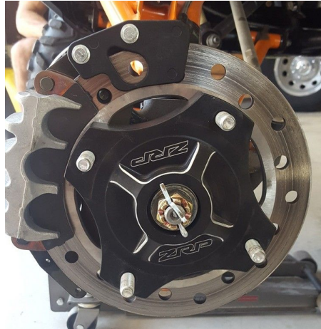
Figure 16: Hub Mounted Disc Brake [8]
