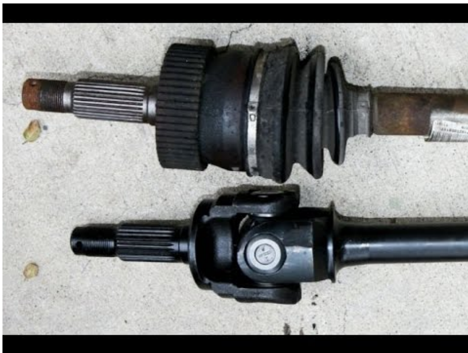
Figure 6: CV Joints vs. U-Joints
