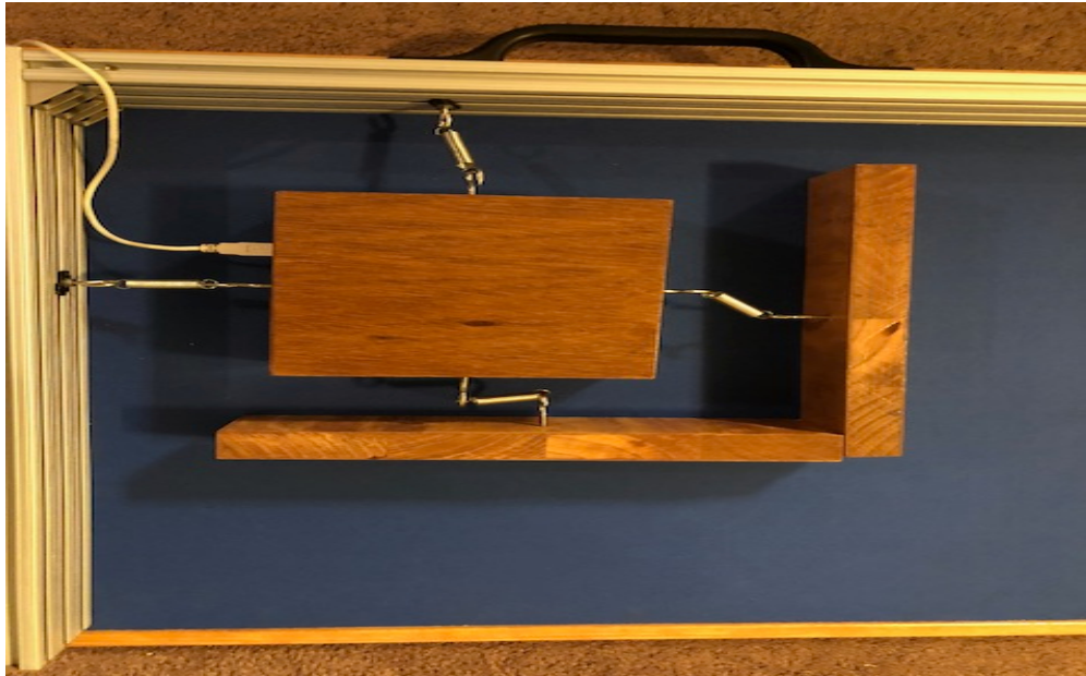
Figure 33: Final system from the top shows all the springs and the blocks
