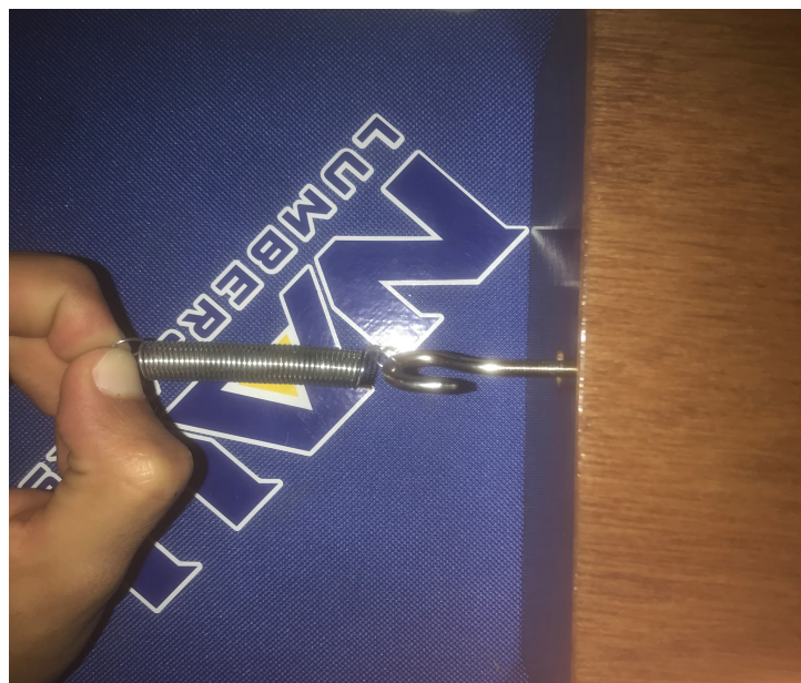
Figure 39: Expanded Spring in same position due to friction
