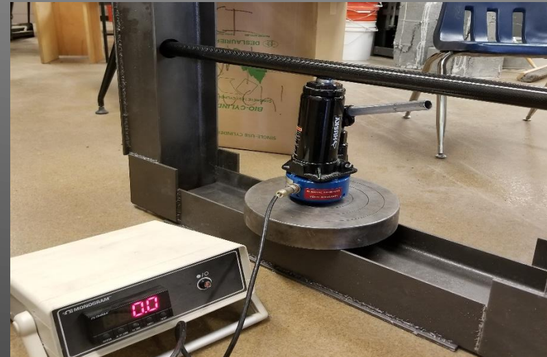
Figure 20. Flexural testing on a test section of HM carbon fiber
