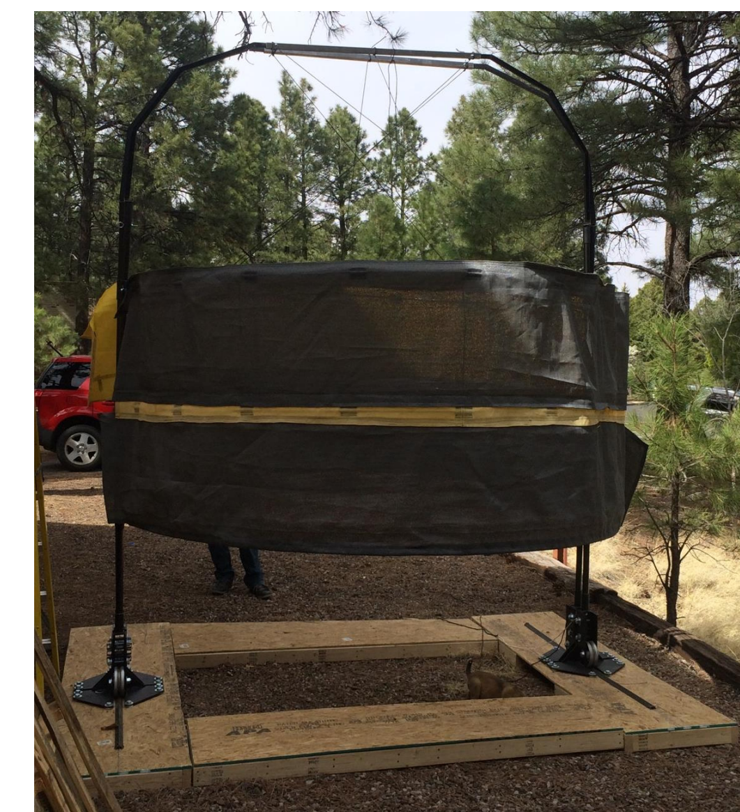
Figure 3. Actual deployed 1/6 scale enclosure with partial water-resistant fabric skin deployed.
