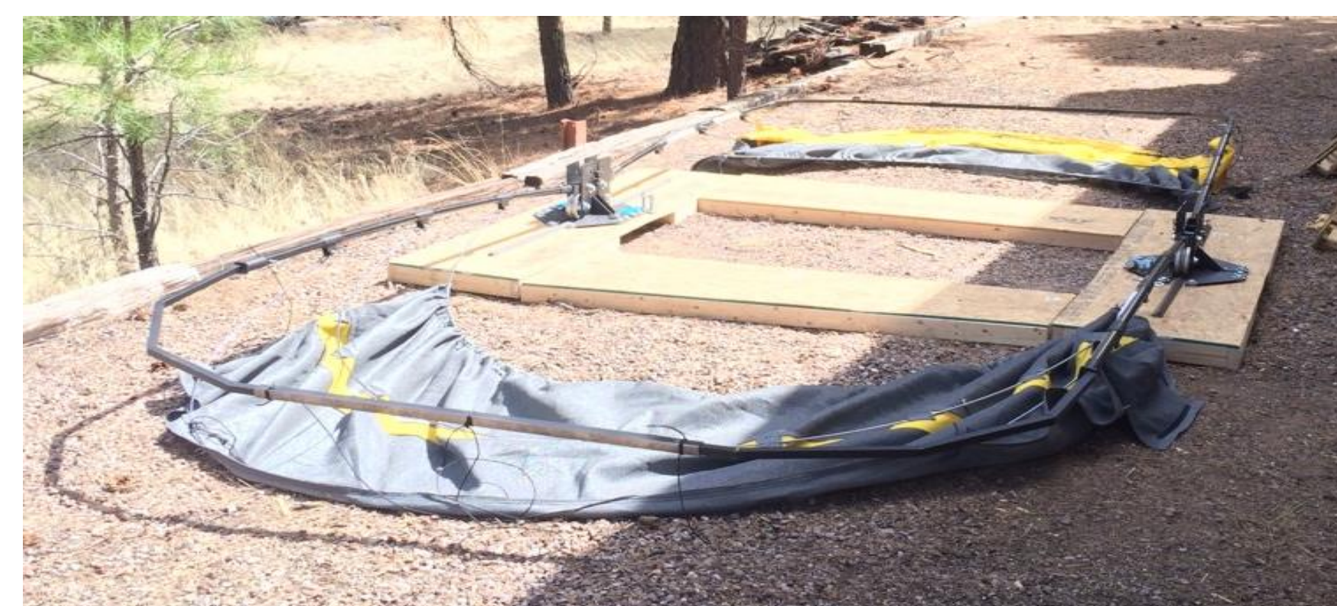
Figure 4. Actual 1/6 scale enclosure in the undeployed position.
