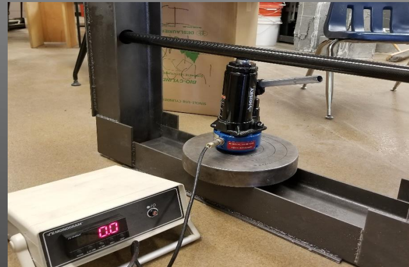
Figure 18. Flexural testing on a test section of HM carbon fiber
