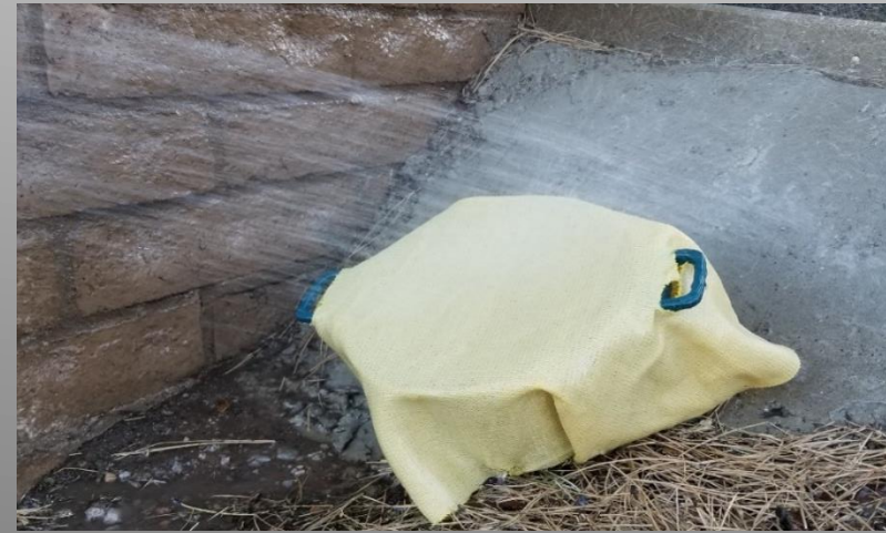
Figure 17. Permeability testing on a test section of HDPE fabric
