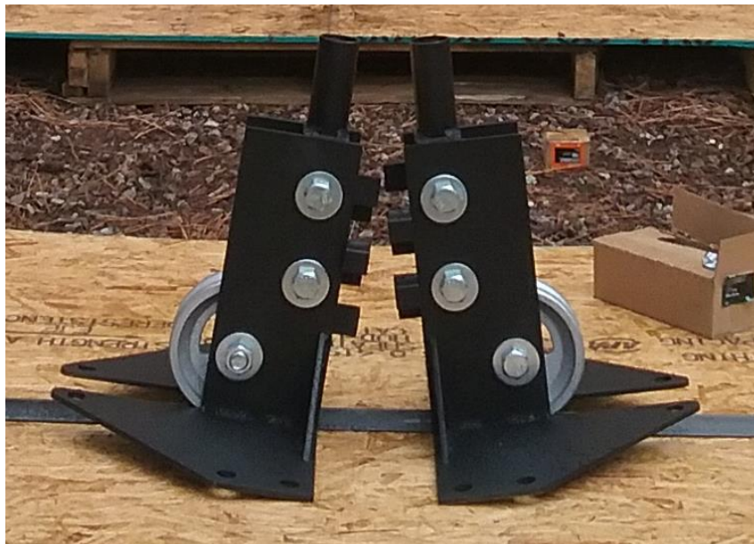
Figure 3: Two base plate halves on v-track
