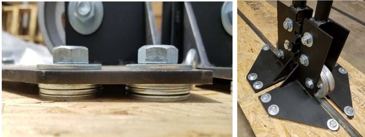
Figure 12: Base plate assembly with washers on left. Secured base plate on right.
