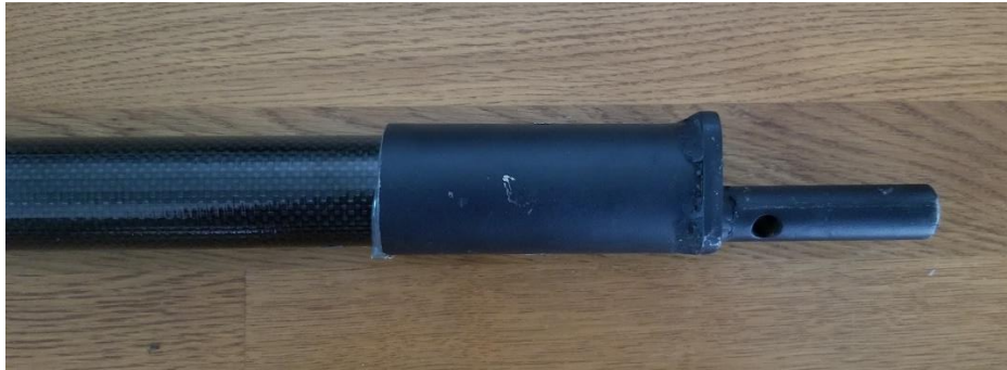
Figure 6: 1.5-foot carbon fiber tube with top adaptor
