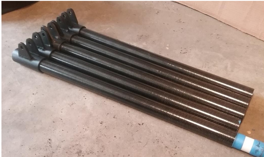
Figure 5: Two-foot carbon fiber tube with hinges
