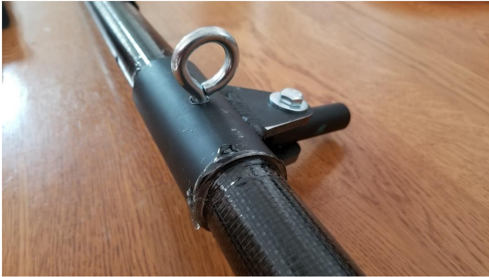
Figure 9: Middle hinge with eyebolt attached
