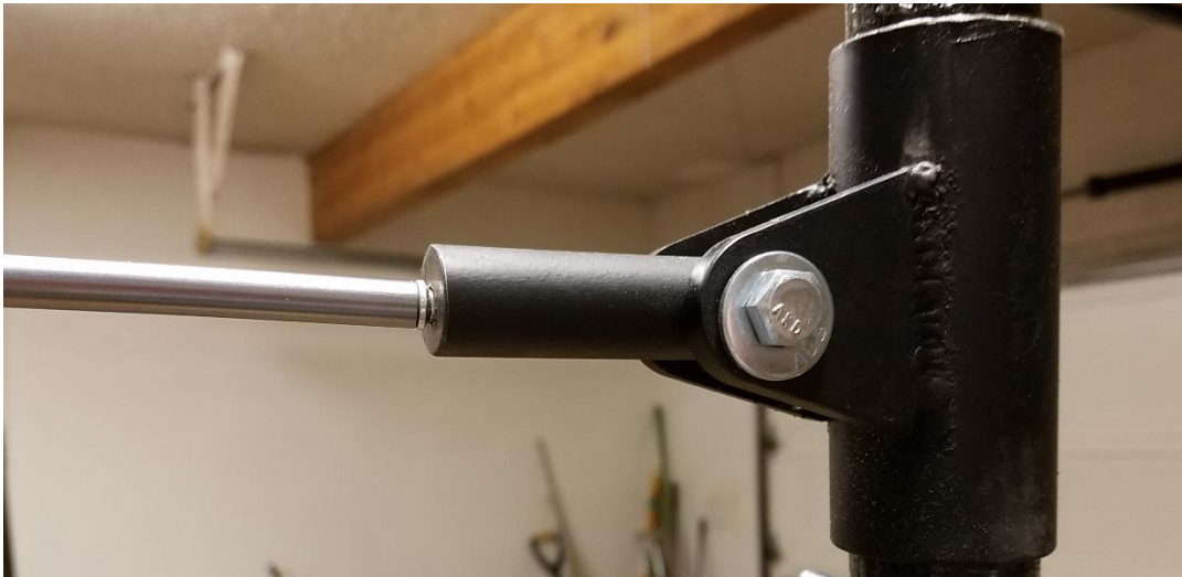
Figure 14: Tent pole inserted in hinge
