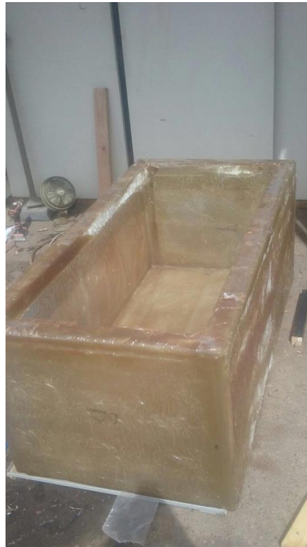
Figure 33: The molded exterior body of the cart.
