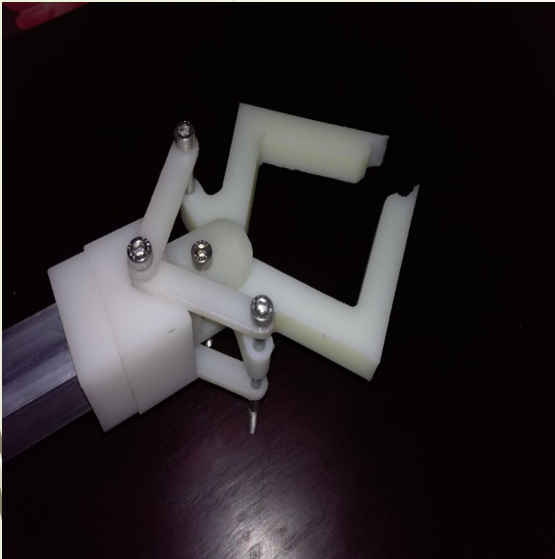
Figure 6: Grabber teeth Hozhoni Assistive Device
