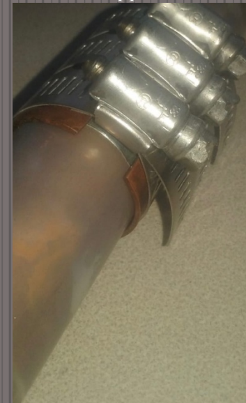
Figure 13: Silicon supported with metal, copper, and clamps.
