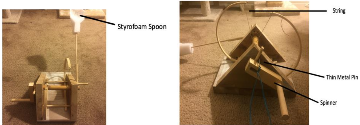
Figure 38: Two different view of the catapult
