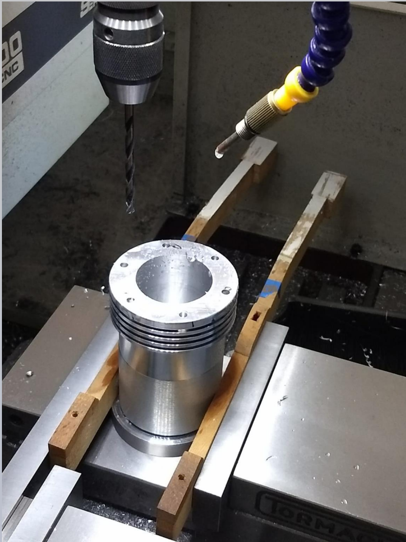
Figure 2. Bolt pattern drilling using Tormach 1100.
