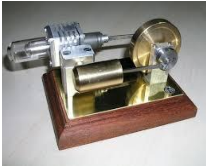
Figure 6. Model of alpha type Stirling Engine [2].
