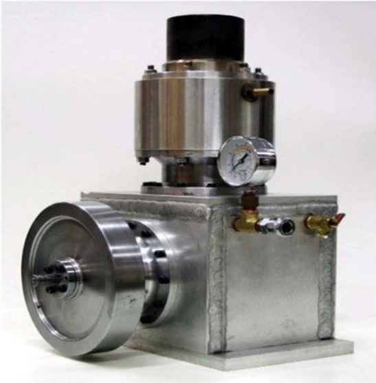
Figure 15 Stirling engine with Scotch yoke drive mechanism
