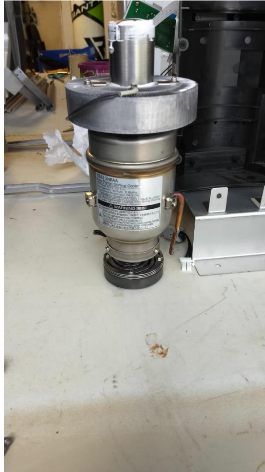
Figure 1. Twinbird Corporation TB42 SN8AA Free Piston Stirling Cooler.
