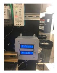
Figure 33. Arduino LCD display housing. Note 24V power supply located in upper left.
