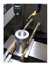
Figure 29. Drilling flange holes with Tormach 1100 CNC. Note: Outer cylinder part with heat fins machined. Finished outer diameter not complete in this photo.
