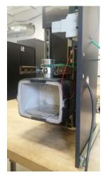
Figure 34. Cooling vessel, Repurposed shelving, adjustable Unistrut, FPSC clamped into position.
