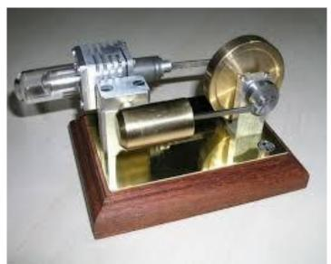
Figure 6. Model of alpha type Stirling Engine [2].
