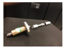
Figure 29. From left to right. Linear motor, motor mount, pressure piston, displacer shaft with collar, displacer piston.
