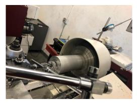
Figure 27. Boring of large diameter raw stock using 4-jaw chuck. Note: indicator dial in upper right of photo.
