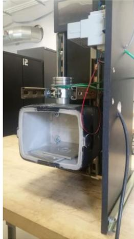
**Figure 34.** Cooling vessel, Repurposed shelving, adjustable Unistrut, FPSC clamped into position.
