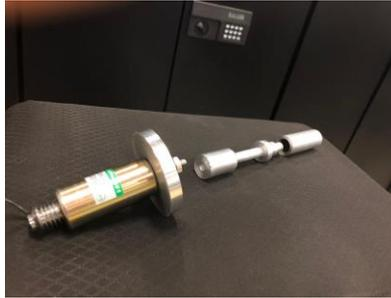
Figure 29. From left to right. Linear motor, motor mount, pressure piston, displacer shaft with collar, displacer piston.
