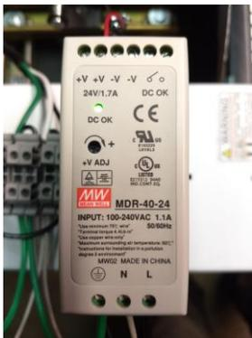
Figure 30. 120 VAC to 24 VDC power supply.
