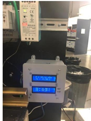
Figure 33. Arduino LCD display housing. Note 24V power supply located in upper left.
