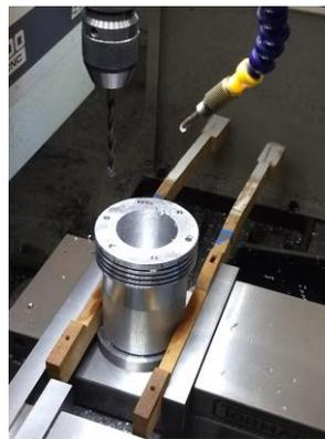
**Figure 29.** Drilling flange holes with Tormach 1100 CNC. Note: Outer cylinder part with heat fins machined. Finished outer diameter not complete in this photo.
