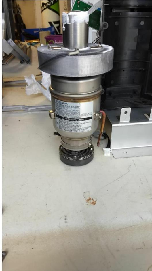
**Figure 1.** Twinbird Corporation TB42 SN8AA Free Piston Stirling Cooler.
