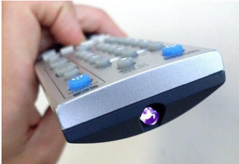
Figure 12: Infrared remote control [10]
