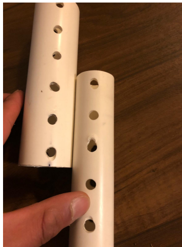
Figure 39: The holes that were made on the PVC pipes
