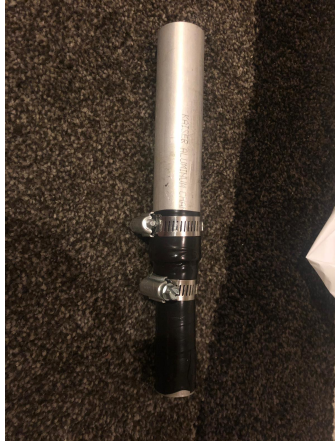
Figure 29: Aluminum pipes with clamps
